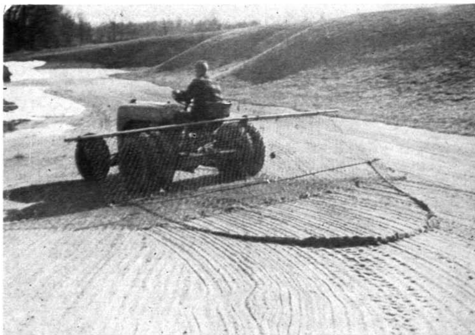
Bunker-raking apparatus devised by T. T. Taylor for use at the Tamarack Country Club, Greenwich, Conn., where he is superintendent.
