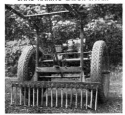
Nelson Monical keeps bunkers raked with little or no hand labor at Portage Country Club, Akron, Ohio. The Worthington Overgreen has solid steel bars welded to the frame to form a rake which does an excellent job. The rake device is easily removed.
