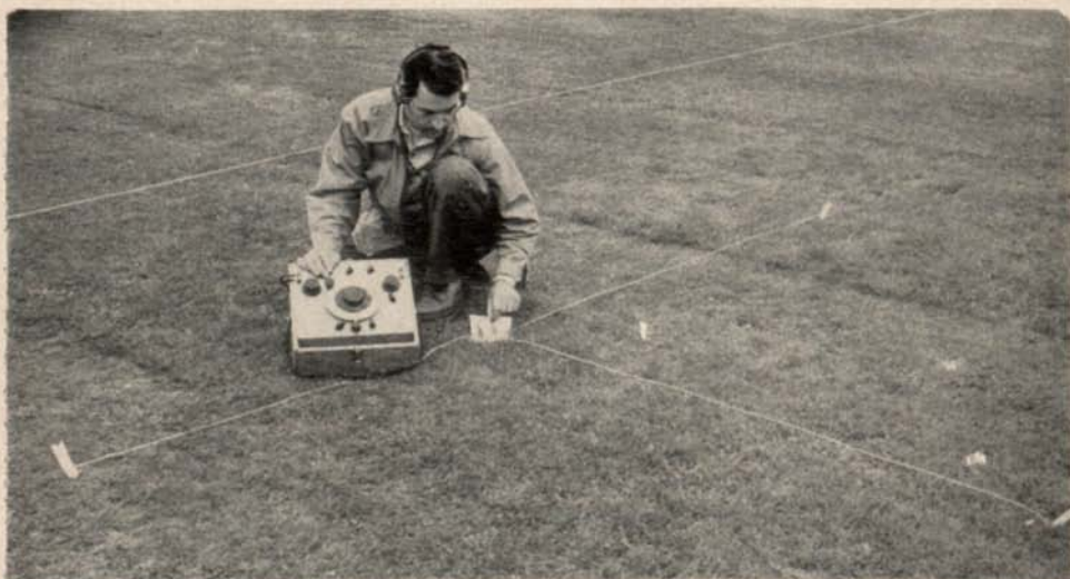
Soil-moisture blocks buried four inches in soil under white arrows were used in irrigation studies at Michigan State College and gave good indications of moisture available to turf through readings on soil-moisture meter shown above.
