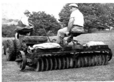
2. Rear view, carrying wheels off the turf. Machine cuts six-foot swath.
