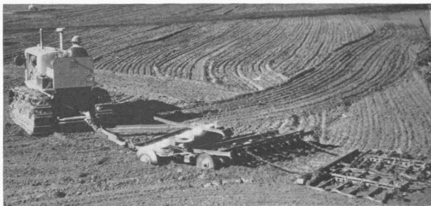
In preparing large areas for turf, a double disk may often be used to advantage. A machine such as this one, having a rear disk which throws the soil in only one direction opposite to the front disk, produces a level seedbed. The spike-tooth harrow dragged behind the disk helps to further pulverize and smooth the soil.
