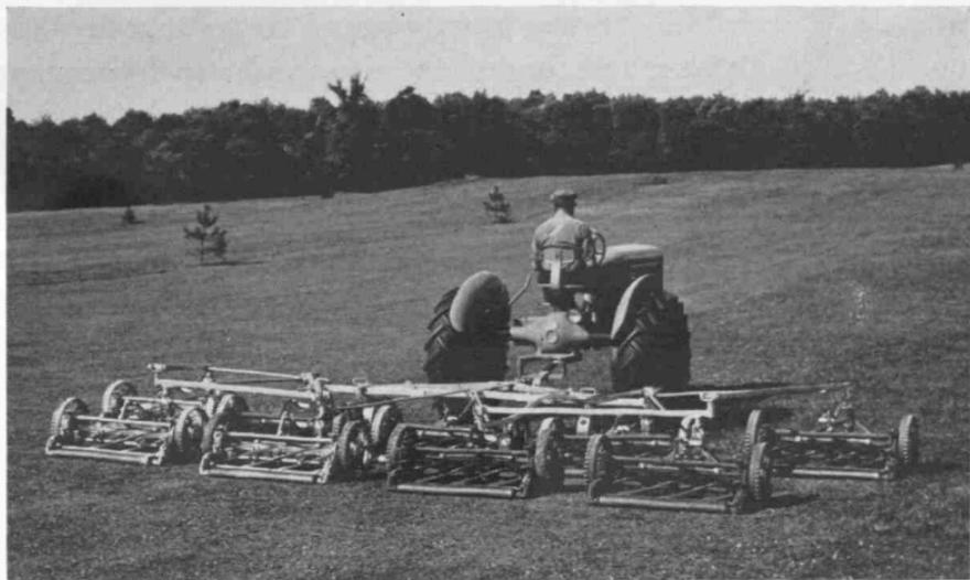
Reel type gang mowers may be effectively used on large open turfed areas. This type of mower is operated at a higher speed and is much more effective in controlling weeds than the ordinary sickle-bar type. The time required for mowing may be kept at a minimum by using 7 or 9 unit gangs of these mowers.
