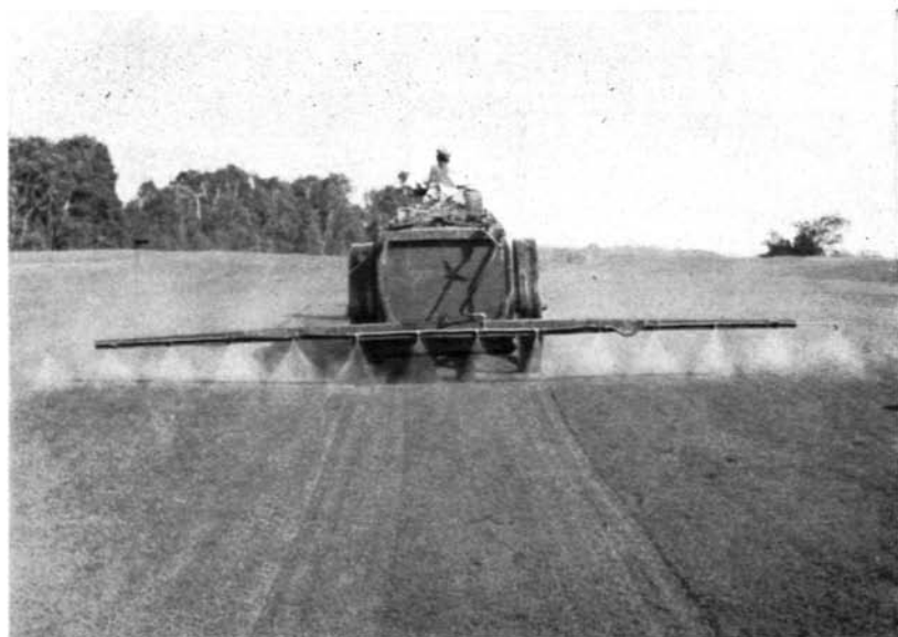
Sprayer showing 20-foot boom with 14 spray nozzles in action.
