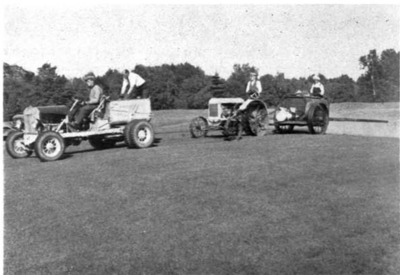
Spraying fairways on Toronto Golf Course. It was necessary to use an extra tractor to operate the pump, as there was no motor on the sprayer.
