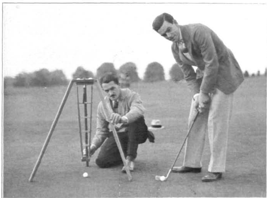
Johnny Farrell, of the Quaker Ridge Golf Club, Mamaroneck, N. Y., National Open Champion in 1928, tests the putting qualities of one of the grasses at the Arlington turf garden, Arlington, Va. The mechanical putter used to eliminate the personal factors in making the tests of drift and speed of the grasses is also shown.
