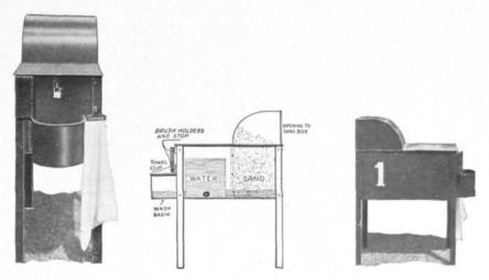
A new, patented tee box, which it is claimed will automatically keep the sand at a uniform degree of moisture. The capillary attraction of the sand on the water is the effective principle employed.
