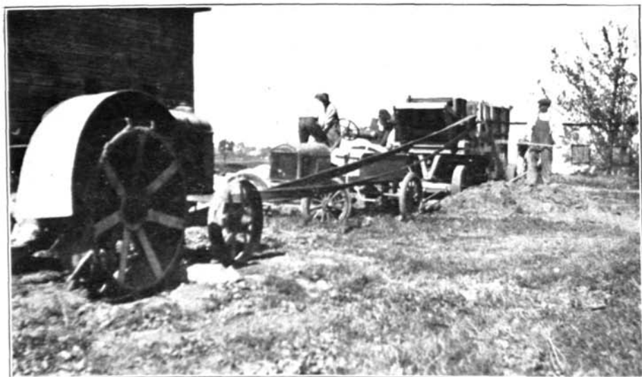
Figure 1. Threshing machine belted to tractor
