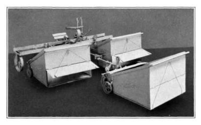
On both ends of the shaft are the ratchets, or pawl cups, in which the pinions operate in conjunction with the ground wheels. The rake heads are divided and hinged, and supported by flat steel springs, to prevent breakage to them or injury to the turf, when any foreign substance is encountered. In each pinion are two pawls, working independently, and the machine can be driven from either side. The rakes are 3 feet wide, thereby giving, with the overlap, a sweeping width of 8½ feet. Our method of
