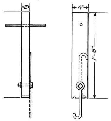
in such manner that it can be lowered for thrusting into the hole to lift the cup and folded back onto the block of wood when not in use for such purpose. The edges of the block at the hook end are chamfered so as to engage the rim of the cup when pressing it into the new hole. When the hook is folded back the block may be used for tamping the earth back into the hole.
