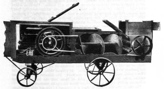
The advantage of the force-feed is that the machine will screen wet, soggy, or lumpy material, whereas, without a force-feed, when the material is wet or soggy the screens will clog, working freely only when the material is fairly dry. The machine is operated by a 3 H. P. gasoline engine.—
