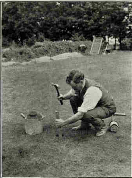
Figure 4—Tamping soil into the old hole
