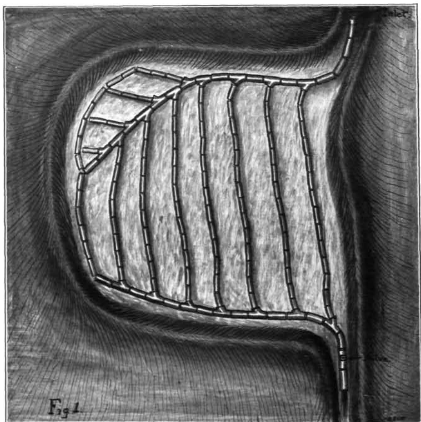
Plan of sub-irrigation system of No. 12 putting green, St. Louis Country Club. The main tile are 6 inches in diameter and the laterals 4 inches
