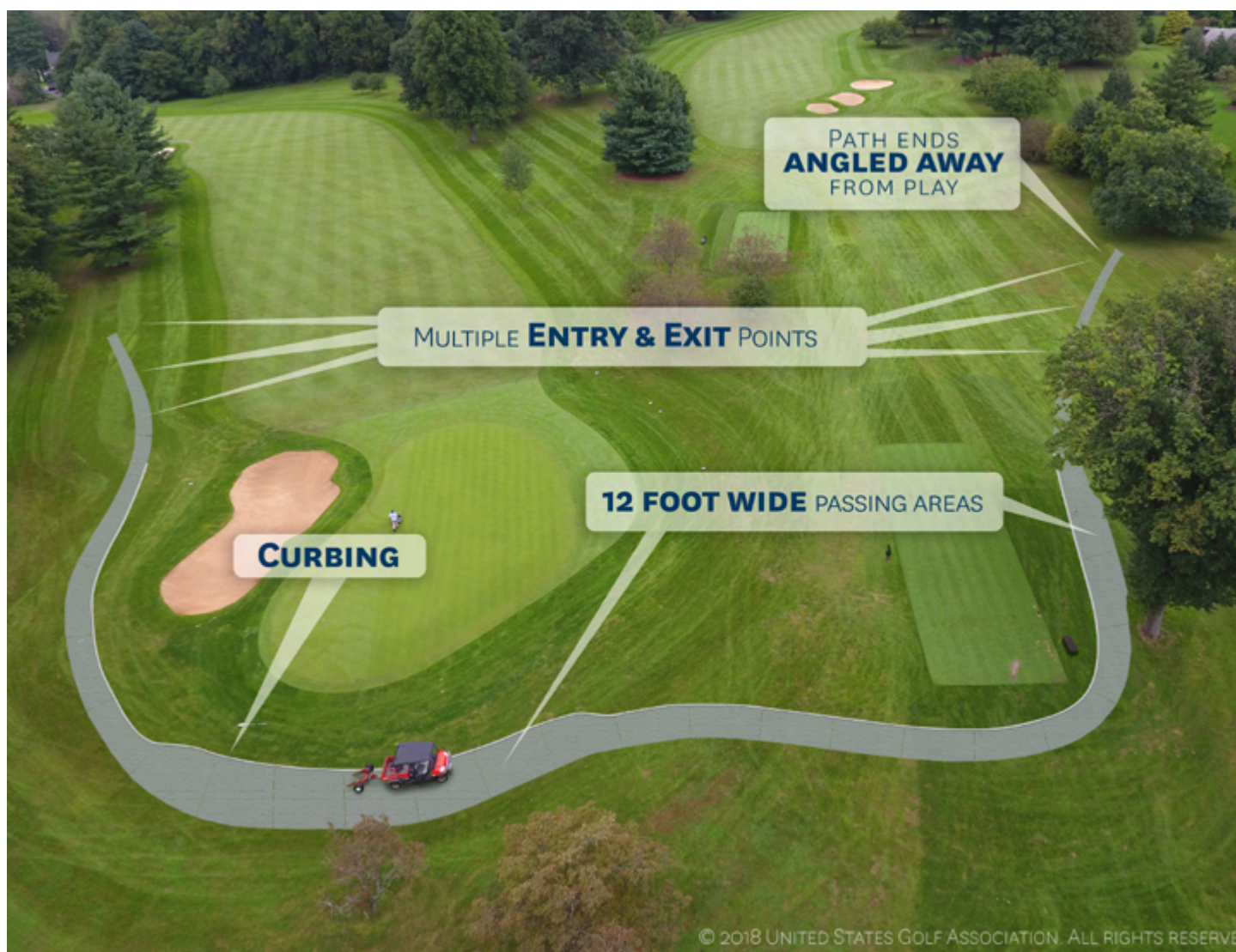
Figure 1. Wrapping cart paths around greens and tees allows golfers to utilize multiple access routes. These areas must be kept free of traffic-funneling obstructions.
