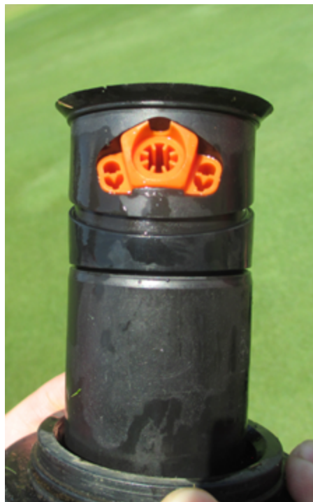
Replacing worn or ineffective nozzles is an easy way to improve the overall performance of an irrigation system.
