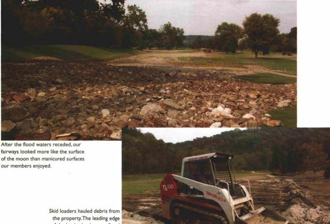
Skid loaders hauled debris from the property. The leading edge of the loader bucket was fitted with a section of PVC pipe to reduce the potential for damage to the turf.
