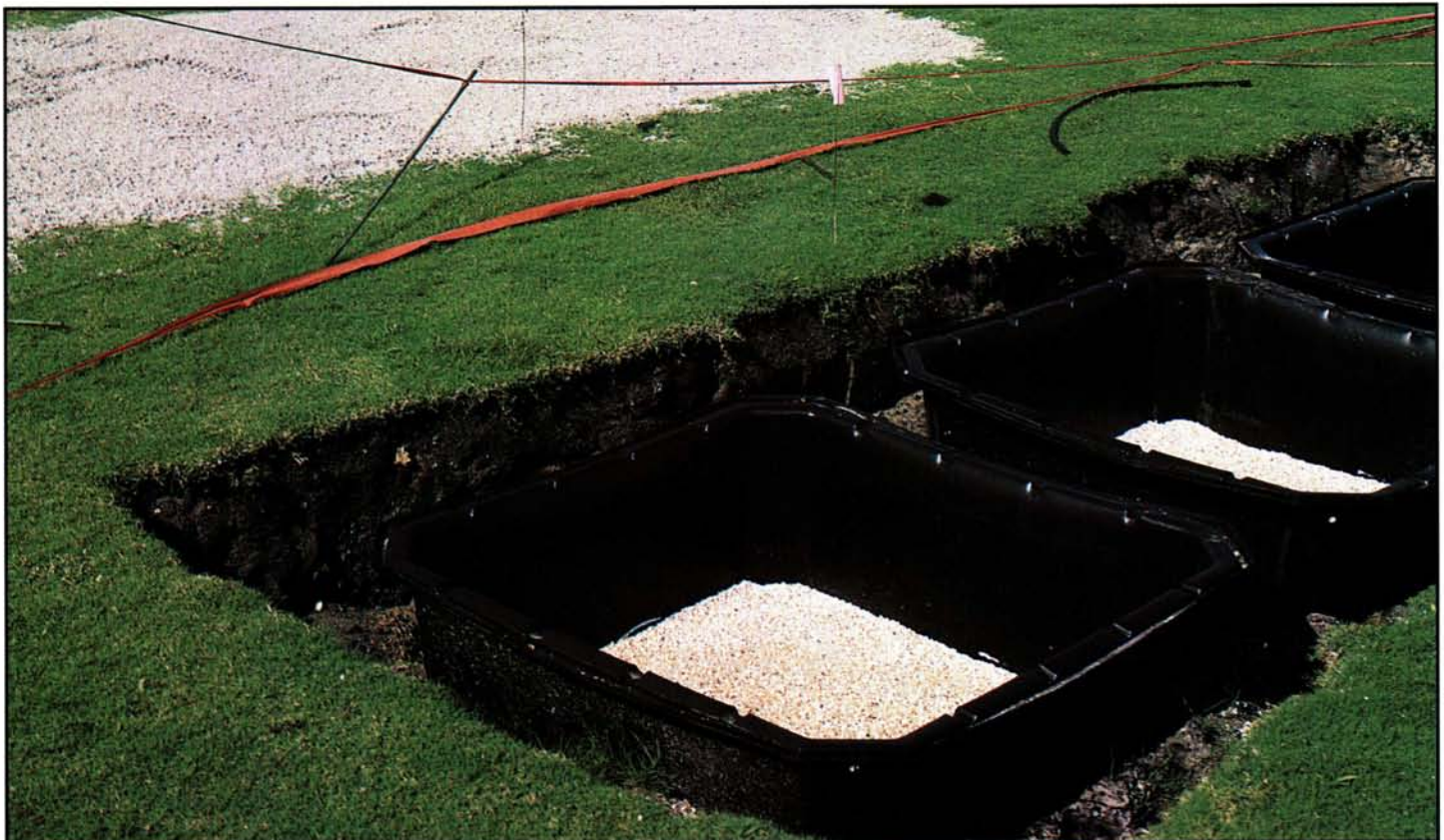
Mini-greens were constructed in 36-inch square, 18-inch deep containers at the University of Florida Research Center in Fort Lauderdale. Soil and turfgrass samples were taken throughout the experiment to determine population sizes of six bacterial groups.
