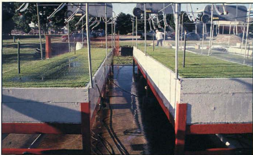
Drainage rates between the two rootzone profiles differed significantly. The USGA profile greens (right) had a higher drainage rate than the California greens (left).
