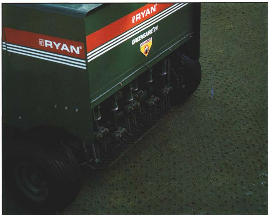
Aerification was used to disrupt the soil surface and prepare the putting green for interseeding a new cultivar.
