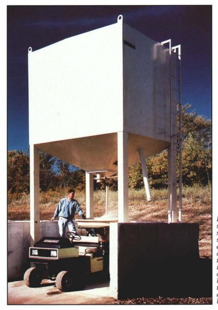
By storing sand in a special silo, one employee can load a topdresser in a matter of seconds by opening the trapdoor at its base.
