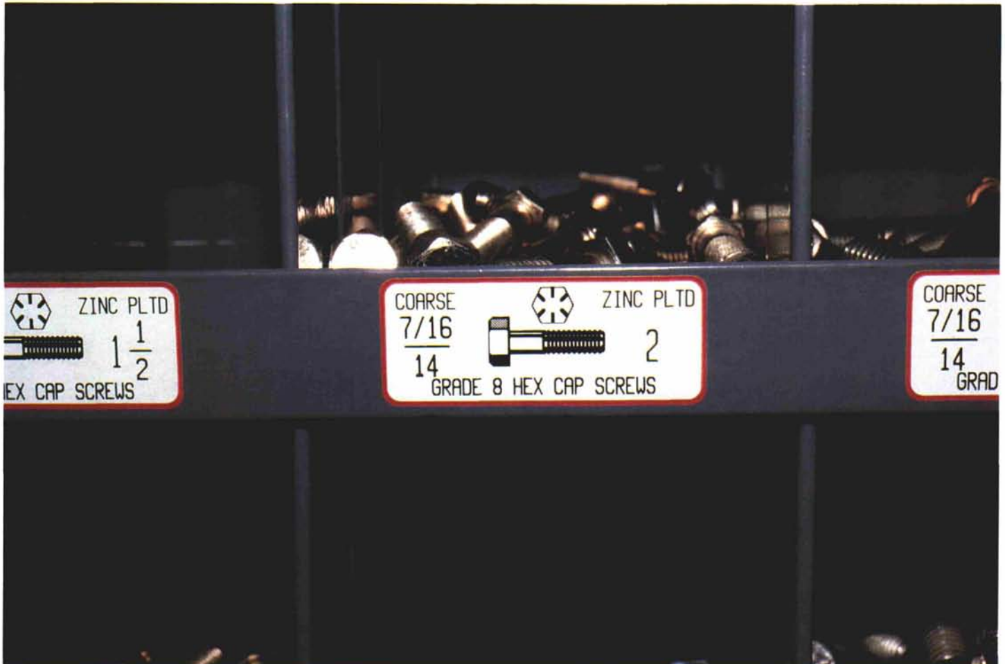
Individual storage bins should be labeled with all the necessary information to make locating a part as efficient as possible.
