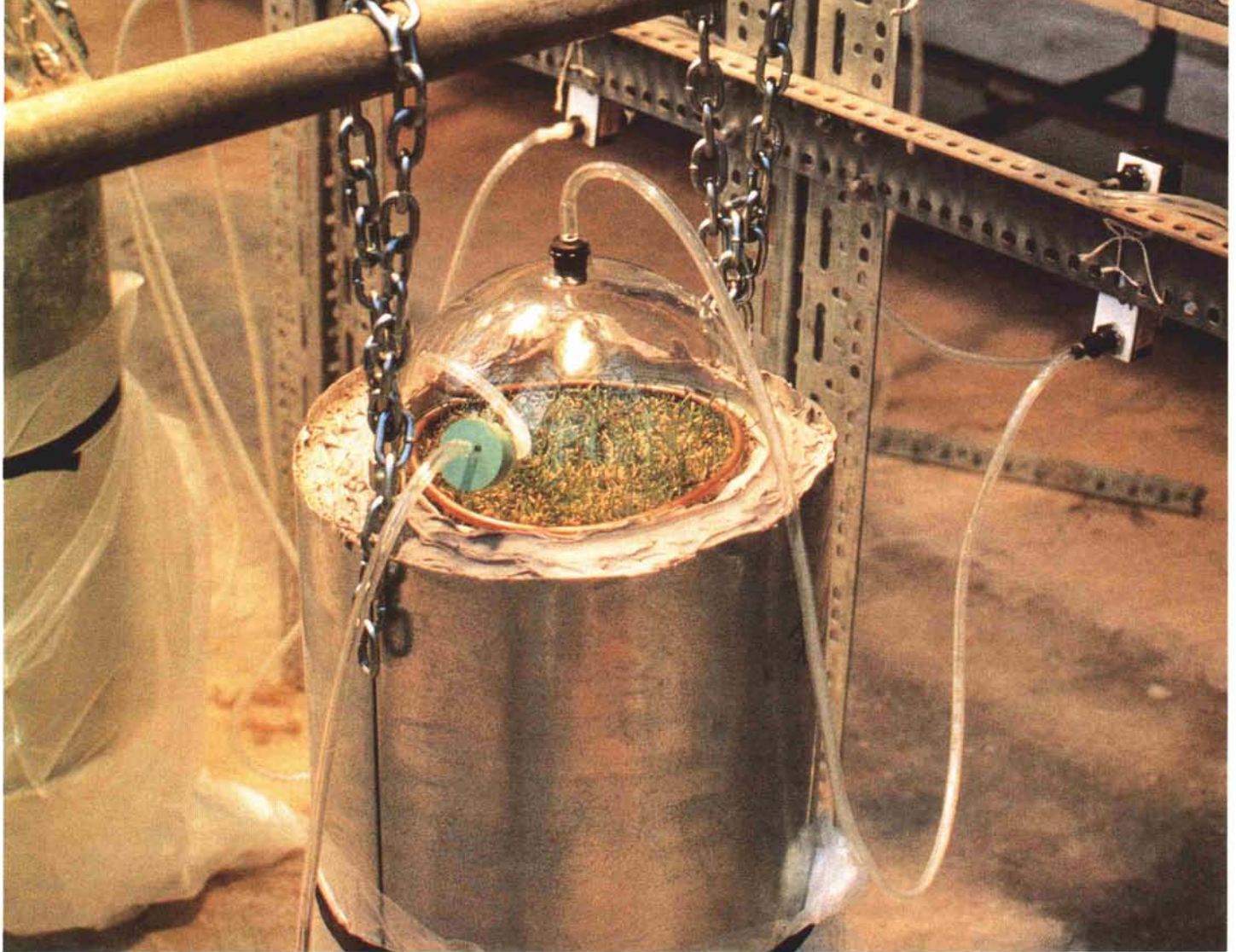
A glass trap system collects volatilized N in the form of ammonia ( \text{NH}_3 ).
