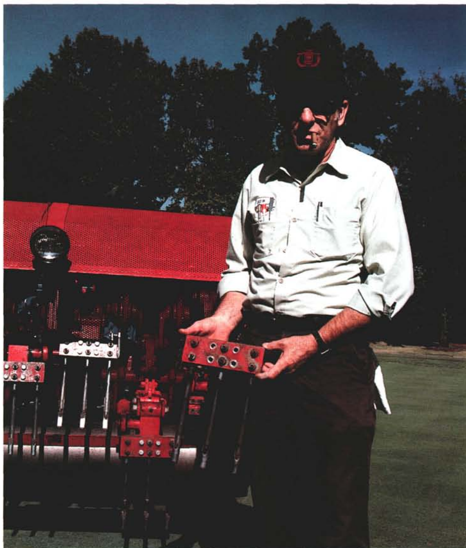
The steel block attaches to the existing tine holders of the Verti-Drain.
