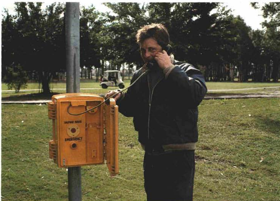
Dave Blasiman, assistant superintendent at Frenchmans Creek Yacht & Country Club, demonstrates the use of this solar-powered, multiple-use emergency/halfway house call box system.
