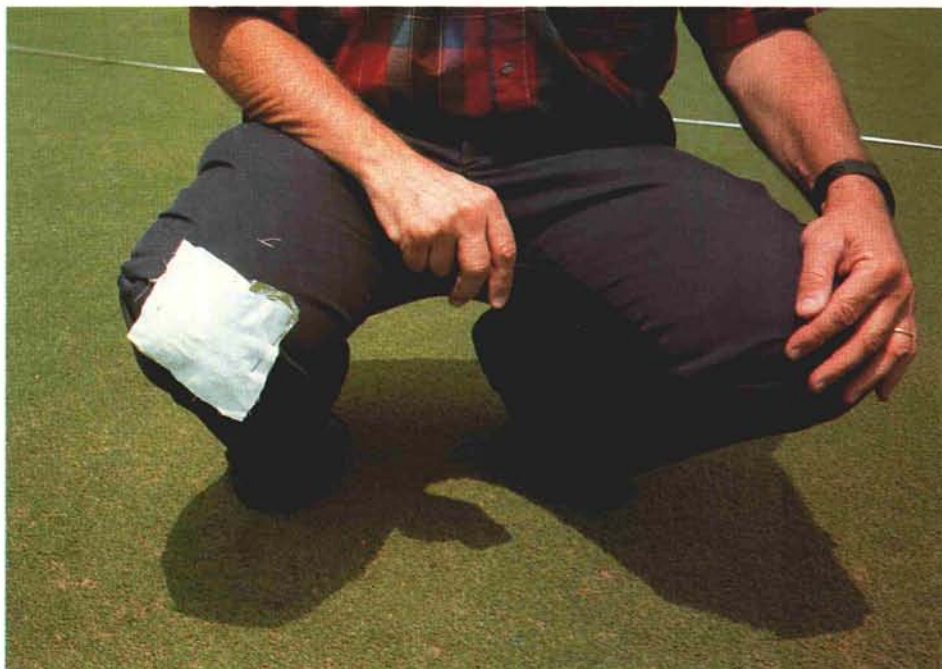
Cotton patches, backed with aluminum foil, were pinned over one knee for tests simulating kneeling while aligning a putt.
