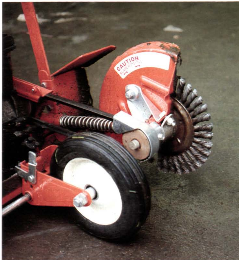
Wire wheel attachments serve as excellent replacements for standard edging blades. The flexibility of the wire wheel produces a clean, uniform cut when edging asphalt cart paths.
