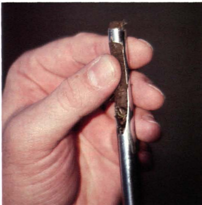
(Above) Knocking the soil probe shaft against your foot will clear out the soil plug and make further probing possible. Be careful where you aim.
