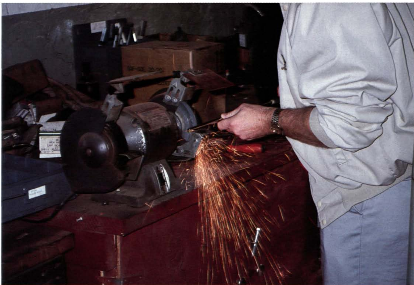
To make a soil moisture probe, a bench-mounted grinding wheel is used to notch out a golf club shaft.
