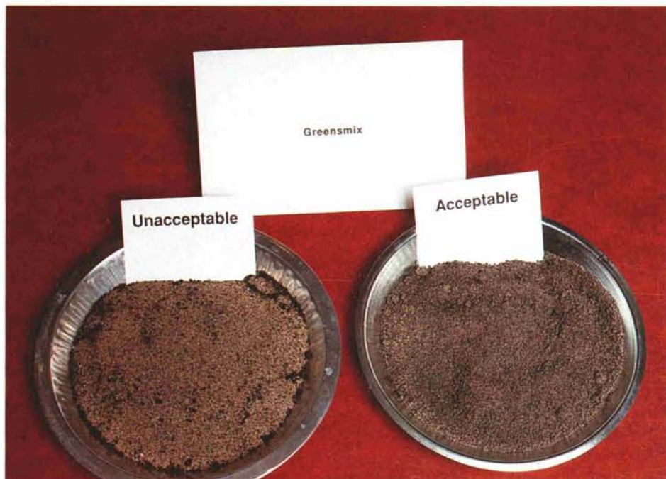
It takes more than a quick look to determine if a root zone mixture meets acceptable standards; it takes thorough testing by an experienced laboratory.
