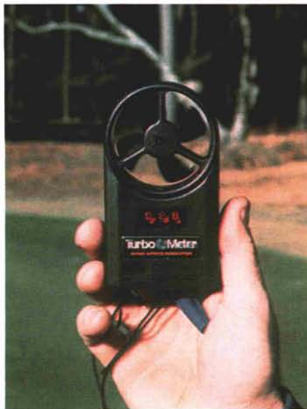
The Turbo Meter, a handy tool to measure wind velocity. The wind speed is in an easy-to-read, digital format.
