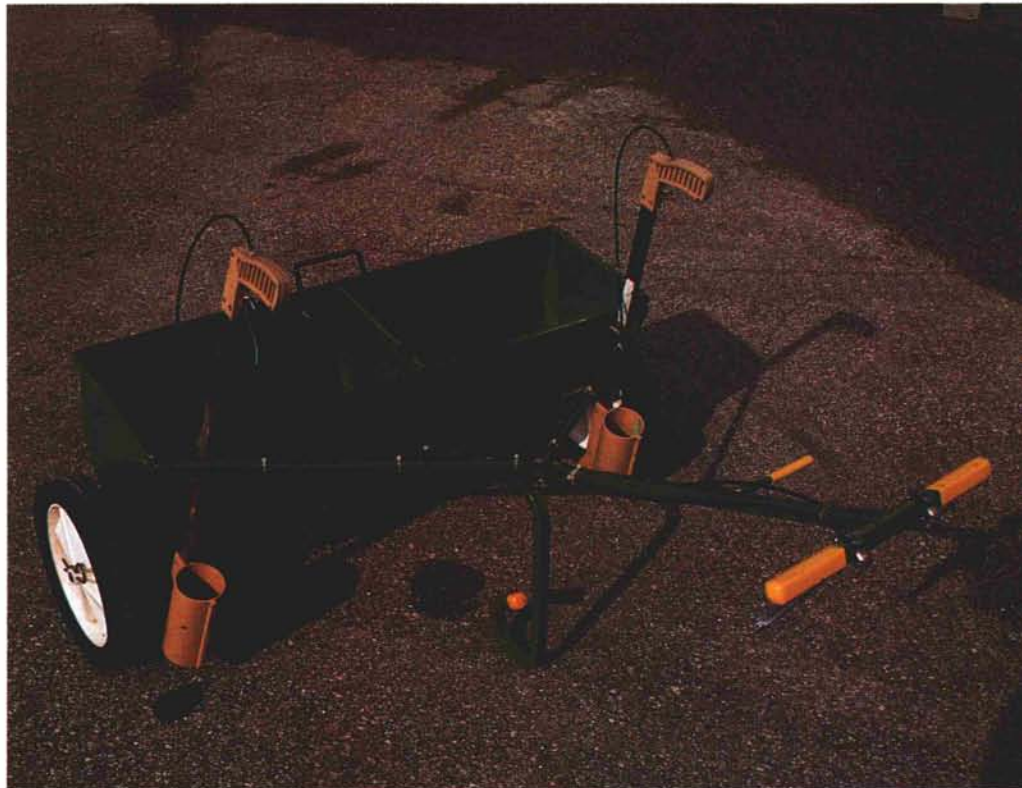
Paint guns mounted on a spreader with bicycle brake handles and cables provide a simple setup for marking where seed has been applied.
