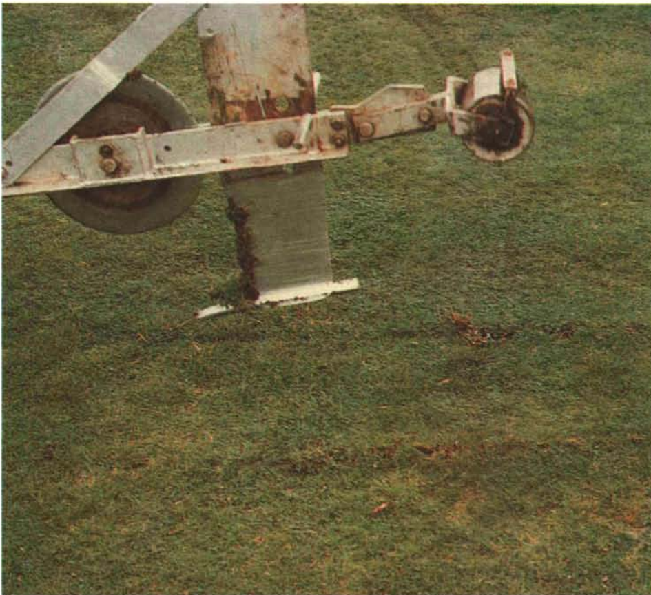
(Top left and left) The oscillating mini-mole plow fractures the soil when a torpedo-shaped device is pulled through the soil. Fissures created by the oscillating mini-moling provide seepage planes for excess water to drain through.
