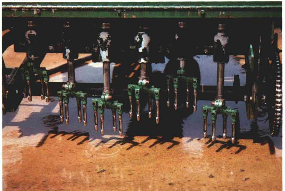
Quadra-tine aeration is an excellent way to improve drainage and "dry out" the turf in a moist, shaded site.
