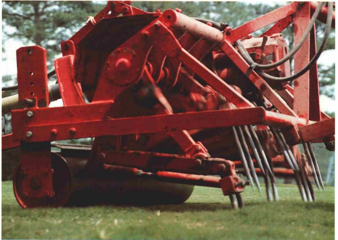
The Verti-Drain uses solid or hollow tines to penetrate the soil 2 to 16 inches for deep soil cultivation of turfgrass sites.
