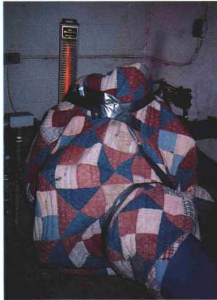
Cover up your irrigation pump to insulate and protect it from a sudden freeze.
