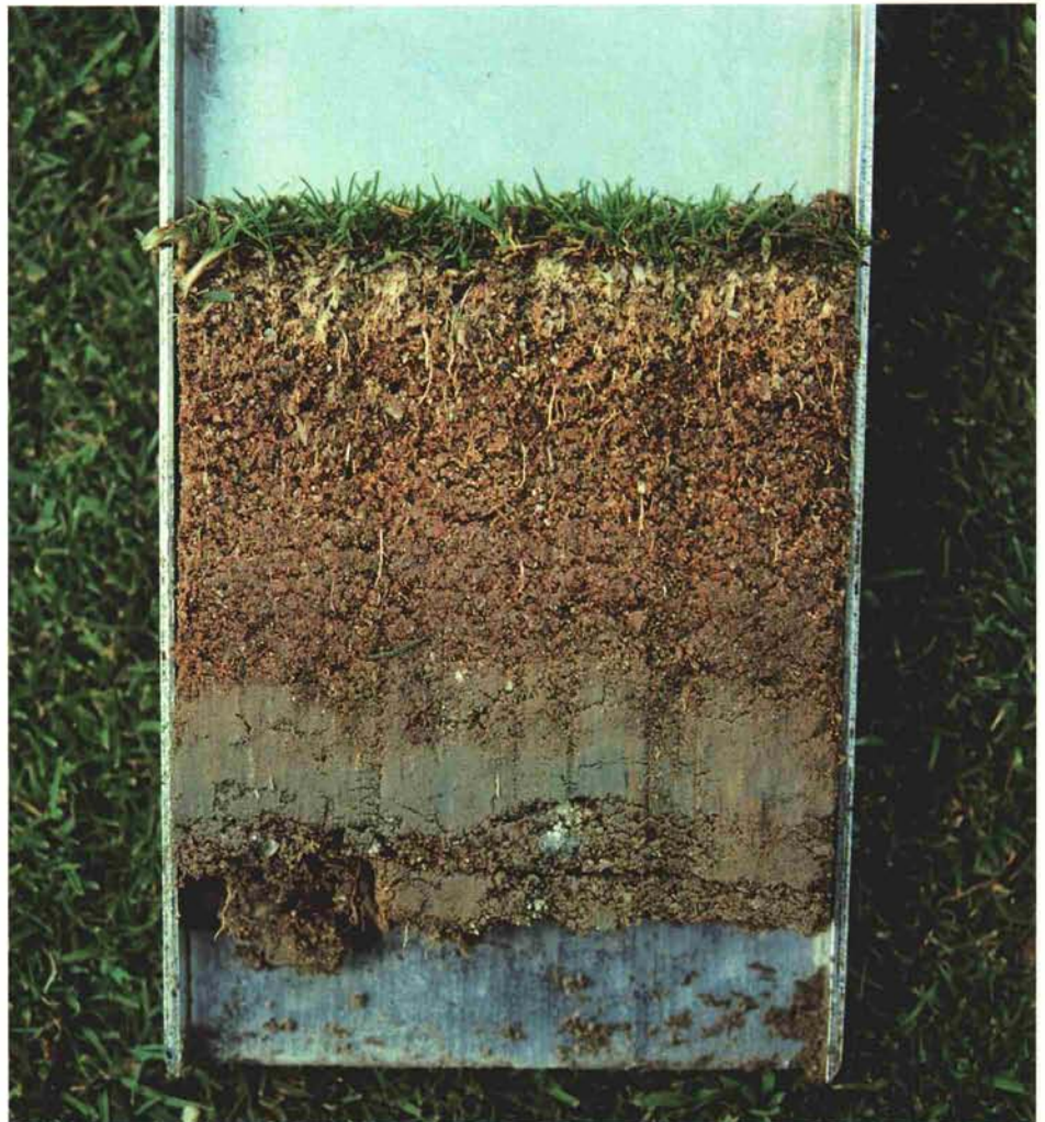
A sand topdressing program established a compaction-resistant growing medium on this green during a five-year period. The green improved significantly and rebuilding was avoided in this case.
