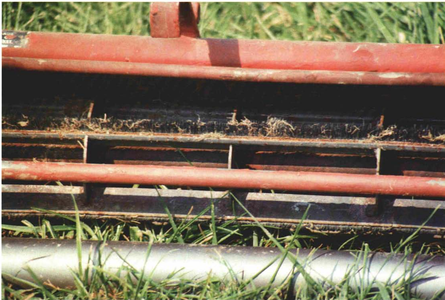
A view of the brush attachment that replaces the cutting blade on the reel.
