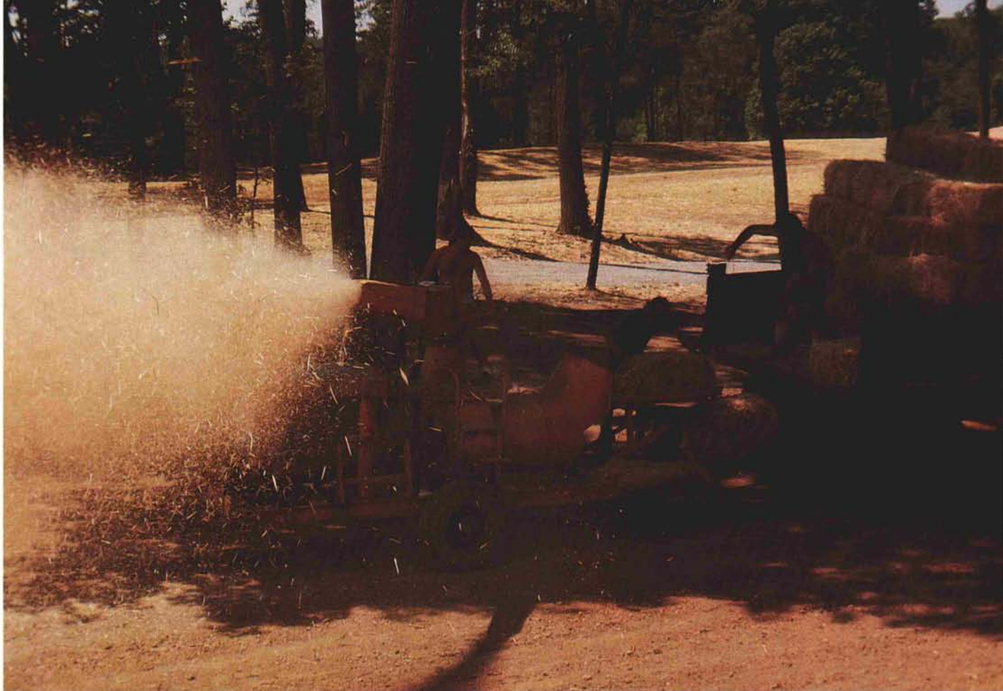
Straw mulching with a power blower.
