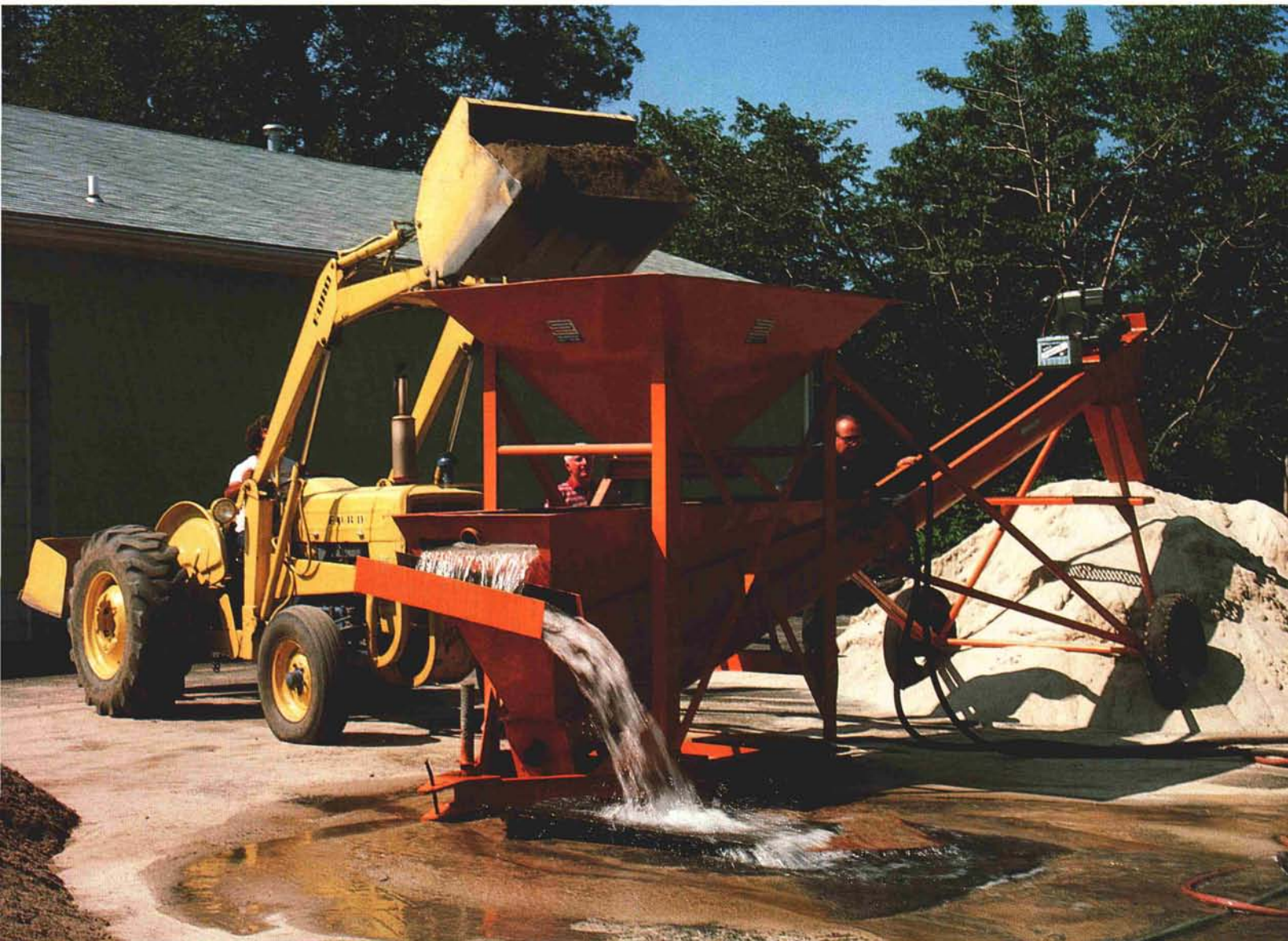
This sand-cleaning machine allows high-quality, expensive sand to be recycled many times. The Country Club of Buffalo, Williamsville, NY.
