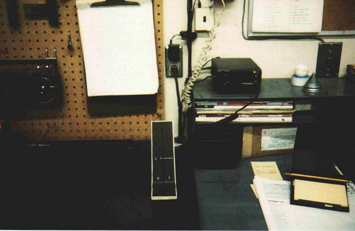
(Left) The base station is equipped with a desk microphone. Usually it is installed in the mechanics' work area.
