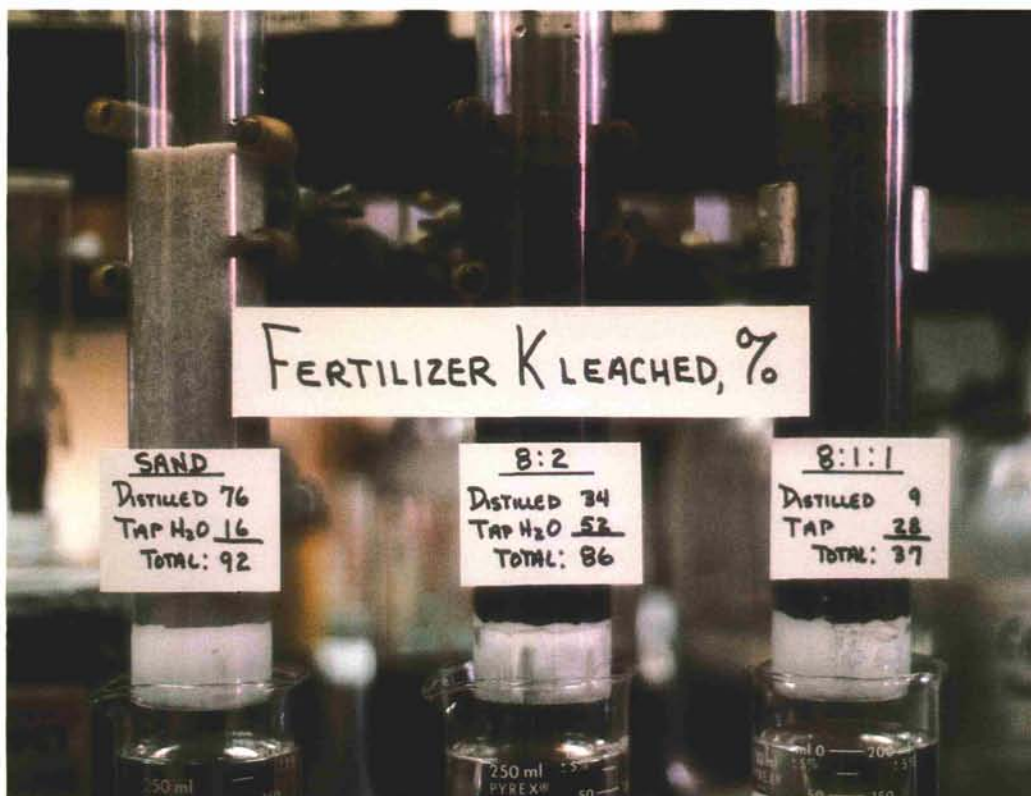
Figure 1: Demonstration of the mobility of potassium in sand, an 8:2 sand-peat mix and an 8:1:1 sand-peat-silt loam mix.
