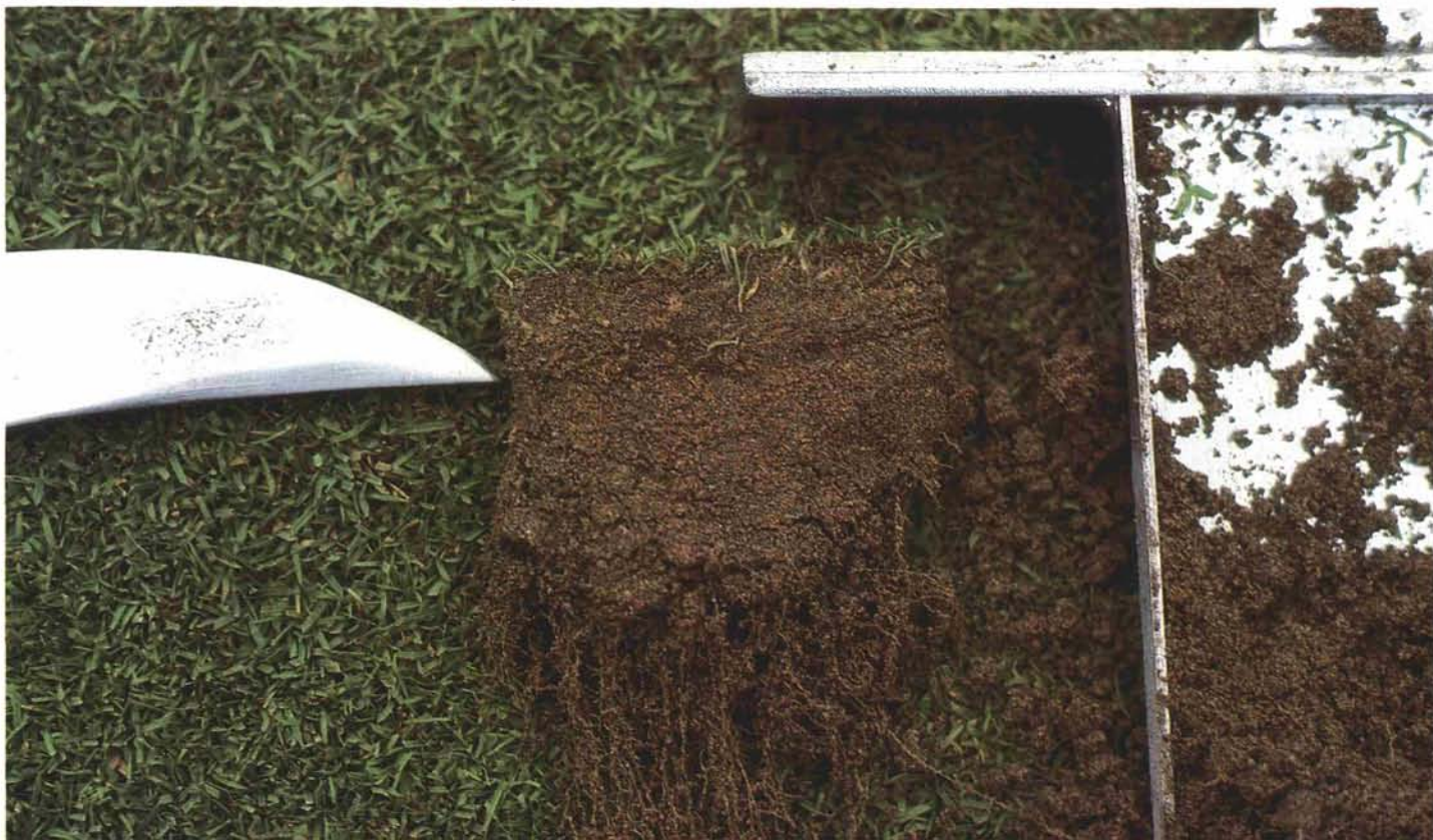
Figure 1: A potential black layer? Excellent root growth in this new green shows strong early turf development. Note the layer of original top growth that was buried by topdressing. This will require spiking or aeration to break up the layer of organic matter before it has the chance to inhibit water movement and become a black layer.
