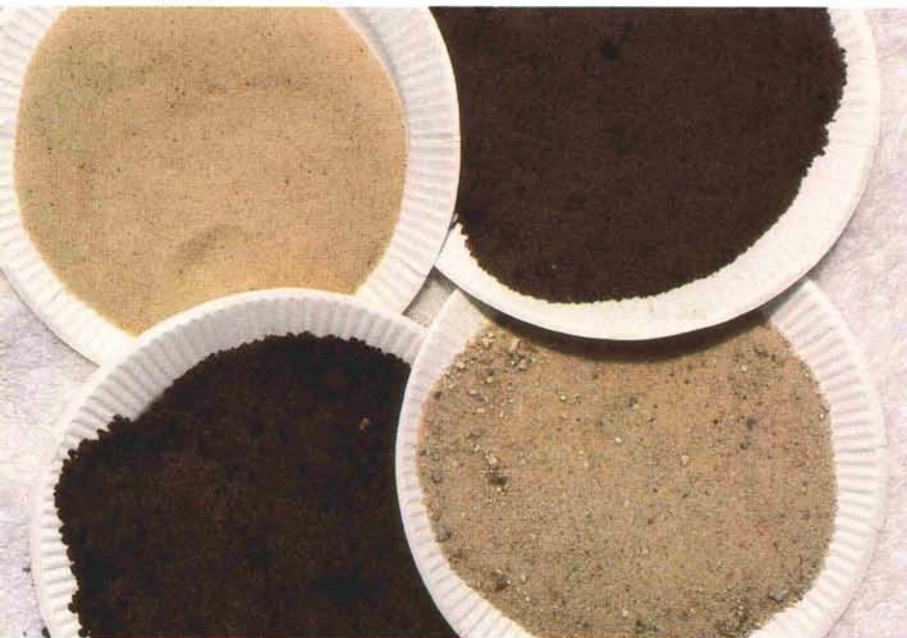
Figure 3: These are four topdressing materials used in 1987, showing a variety of opinions and products: Upper left, well-graded industrial sand, about 76 percent in medium ranges and the rest above 0.15mm. Upper right, same sand with 20 percent peat added. Lower left, same sand with 40 percent soil added. Lower right, a masonry sand. Imagine the quantity of the larger particles that will be removed in dragging and cleanup procedures.
