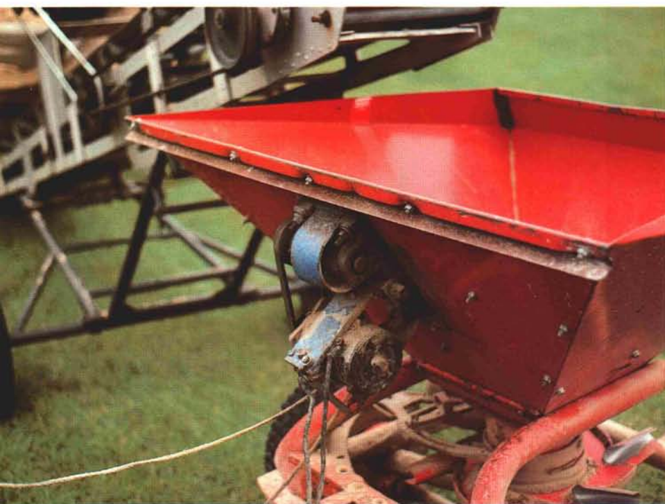
A vibrator is bolted to the broadcaster's hopper, which assures the flow of very wet sand to the spinner at a rate determined by the driver of the towing vehicle.
