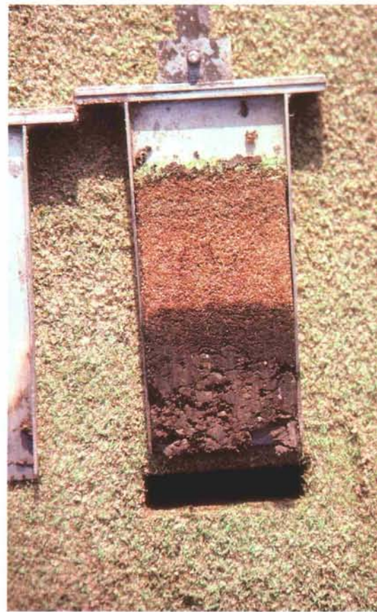
Distinctly different layers in a profile can inhibit root development and water movement.
