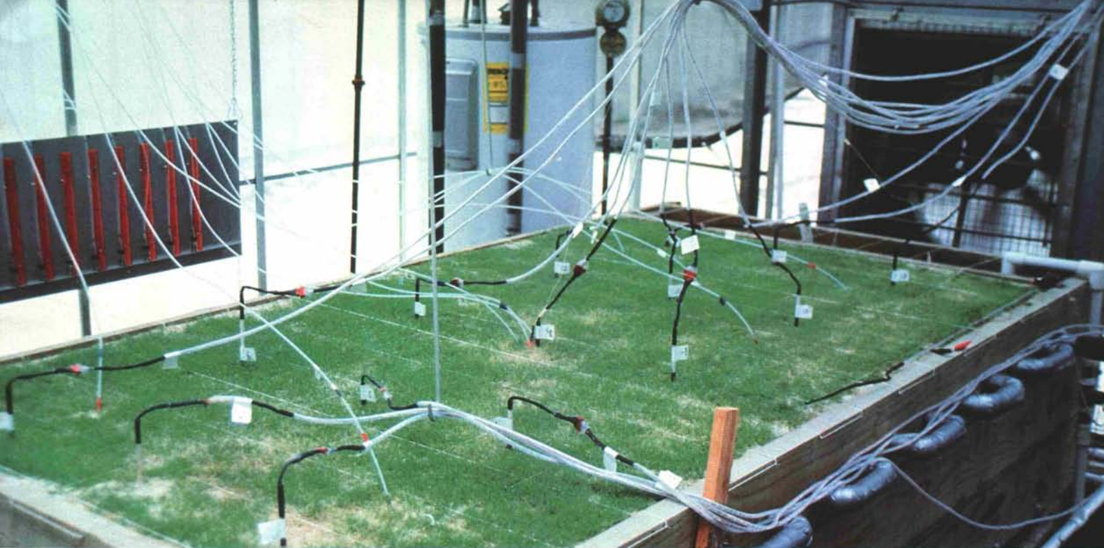
Figure 1. Heat bench to create high soil temperatures, a facility developed to screen large populations of plants for survival under high soil temperature.
