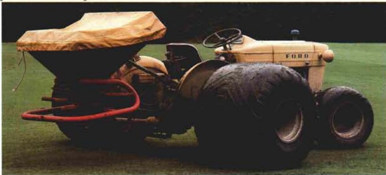
Figure 6. (Bottom) The "big tire" combined with a large-tire trailer is excellent for brush cleanup or soil movement under wet conditions.
