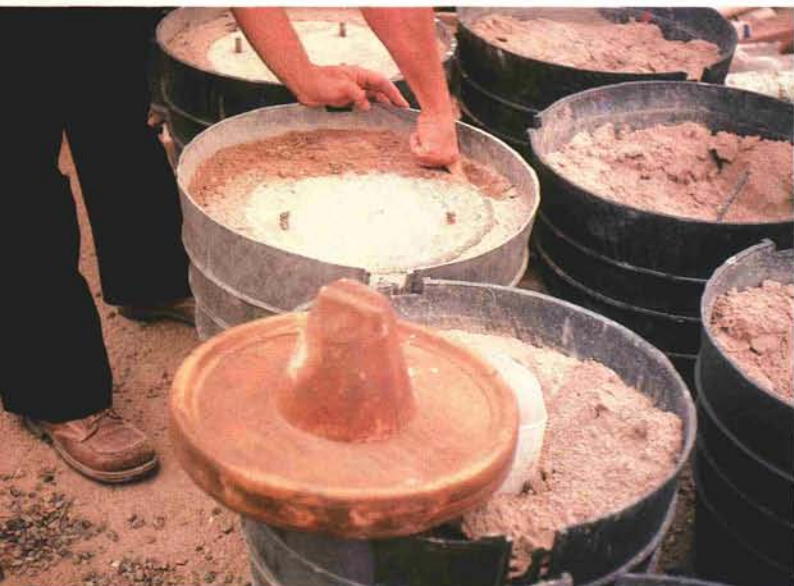
Santa Teresa Country Club, New Mexico, is just a few miles west of El Paso, Texas. Here, using a wooden mold and sand to create a form, they make concrete sombreros for their tee markers. These are then hand-painted with designs for championship, men's, regular, and women's tee markers.
