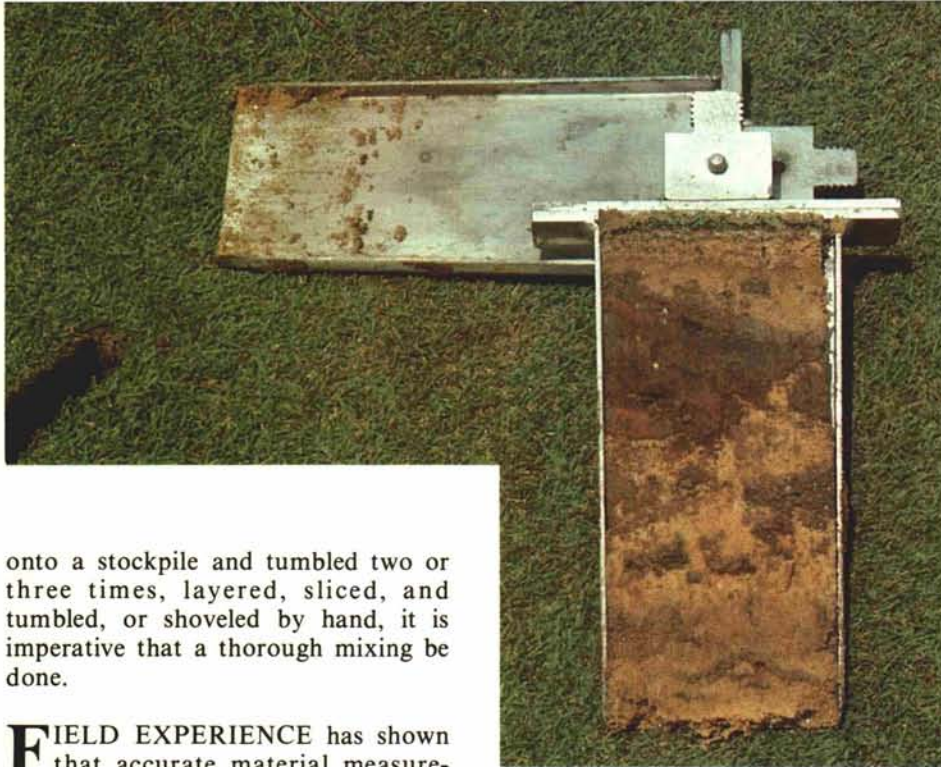
A typical result of on-site mixing: lack of uniformity.
