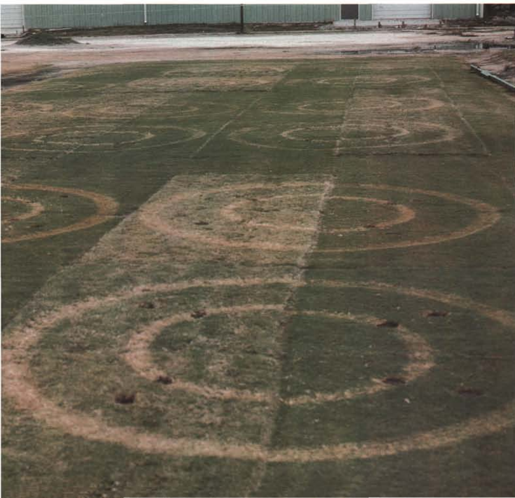
Wear stress simulator test on cool-season grasses at Michigan State University (left) and the wear pattern after use on bermudagrass at Texas A&M University (below).
