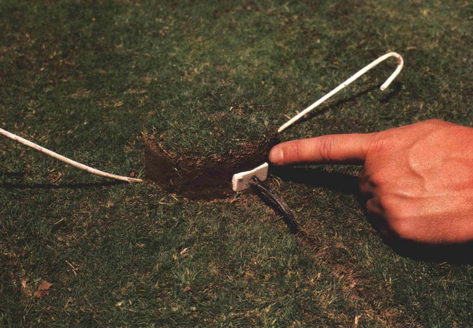
View of gypsum block placed approximately 1 inch deep in the soil to monitor available water during the 1979 growing season. The wire lead is attached to a soil moisture meter.
